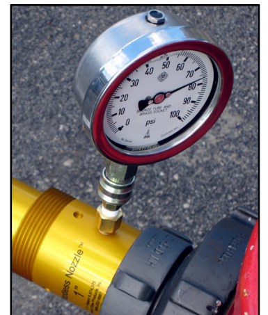
Pitotless nozzle for precise flow rate measurement from 48 – 1,602 GPM
