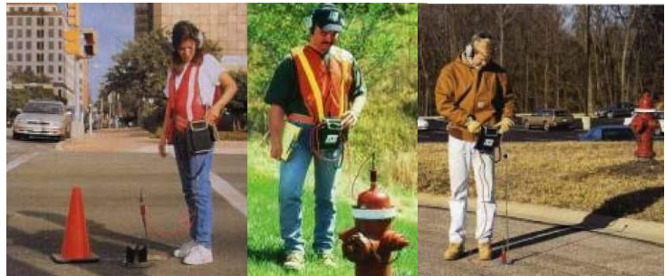
Downtown leak survey on main line valve
